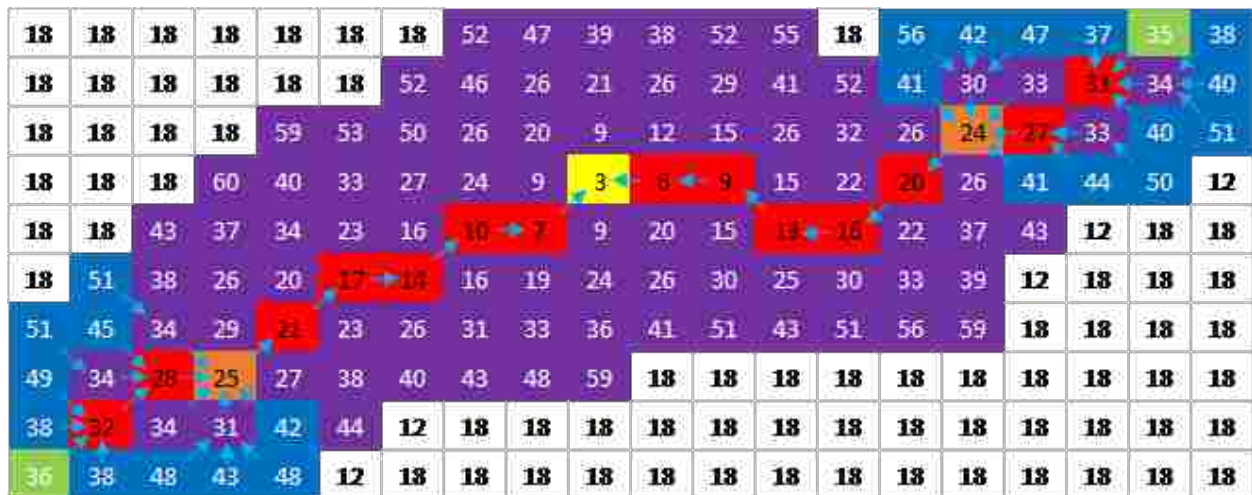
(b) Extending start points in our numerical example. Green pixels (end points) are part of, and complete the (red) optimal path for this image.
